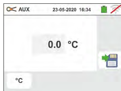
Fig. 33: Measurement of environmental parameters through external probes
