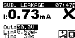
Figure 0.44: Example of substitute leakage current measurement results
