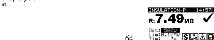
Figure 0.79: Insulation resistance - P result screen
