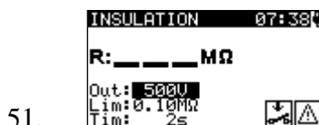
Figure 0.74: Insulation resistance starting screen
