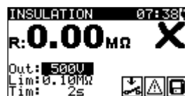
Figure 0.38: Examples of Insulation resistance measurement results
