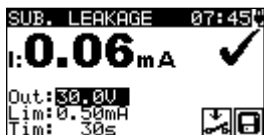
Figure 0.44: Example of substitute leakage current measurement results
