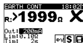
Figure 0.35: Examples of Earth continuity resistance measurement results
