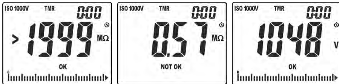
Fig. 21: Results of insulation measurement in TMR mode
