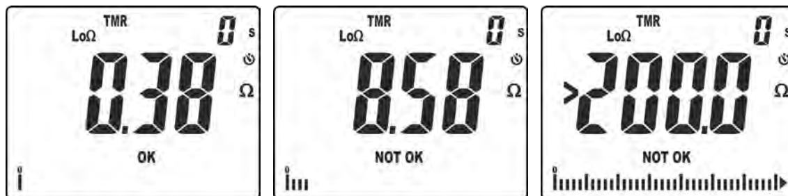
Fig. 31: Results of continuity test in TMR mode
