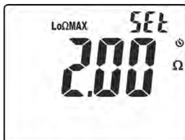
Fig. 26: Setting the limit threshold for continuity test
