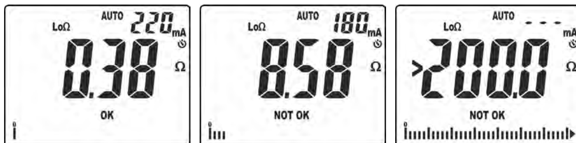
Fig. 28: Results of continuity test in AUTO mode
